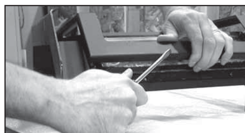
Figure 8.3 Use a flat-head screwdriver to pry the black crown free on the right side. Remove the crown and discard.
