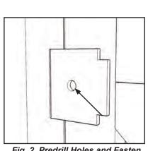
Fig. 2. Predrill Holes and Fasten with S5- 1" Pan Head Screw
