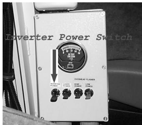
Figure 2.2.5.6. Remote switch for inverter power.
