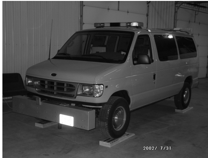
Figure 2.5.4.2. Profiler on top of support blocks.
