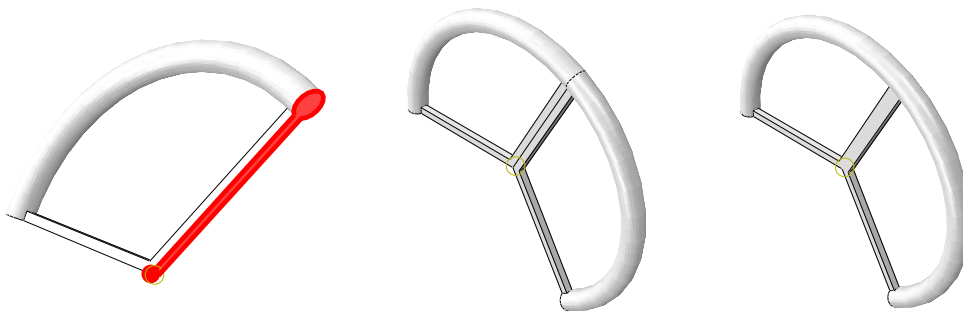
Figure 4–5 Mirror features, with and without internal boundaries.
