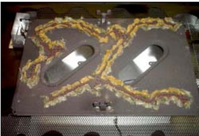
Figure 43 Placement of the Ember Material
