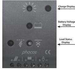
Solar Panel Battery Load Connection Connection Connection
