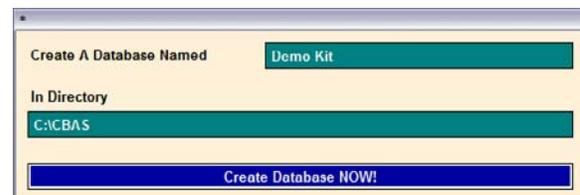
After a short time, the new database will open in Editor Mode/Hardware View. You can now create Channels, Controllers and Points, in that order.
