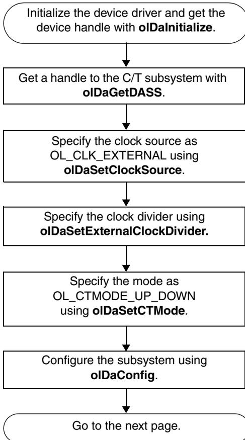
Specify the appropriate C/T subsystem/element. The DT9834 Series supports five elements (0, 1, 2, 3, 4).
