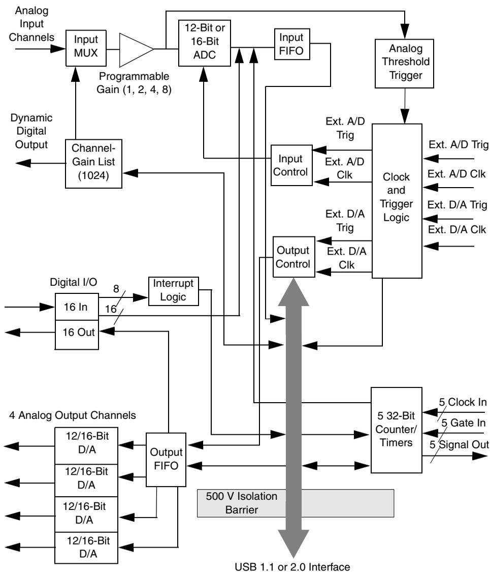
Figure 1: Block Diagram of the DT9834 Series Modules
