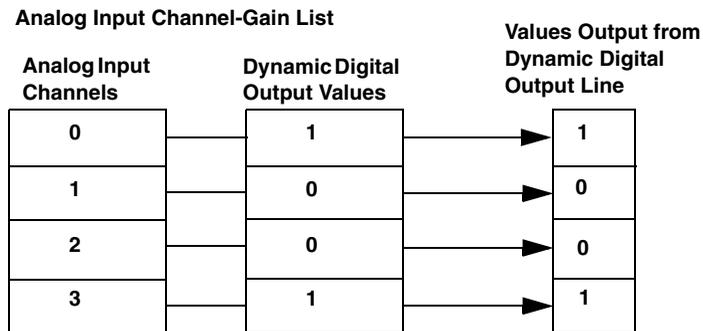
**Figure 2: Example Using Dynamic Digital Outputs**
