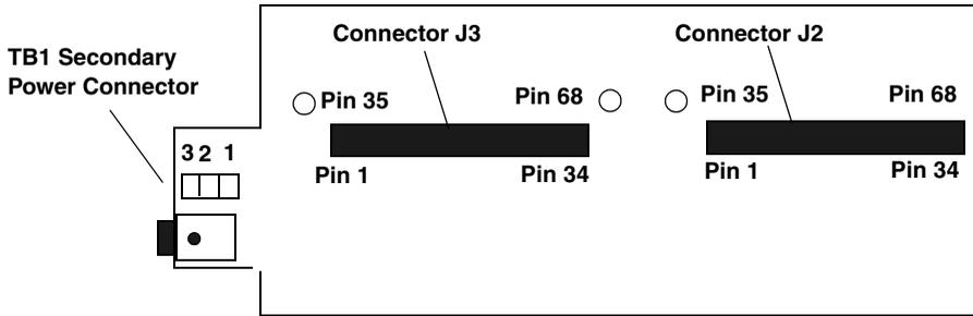
**Figure 6: Orientation of Connectors J2 and J3**
