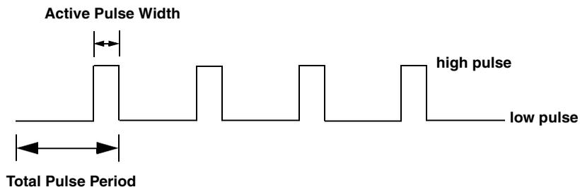
**Figure 5: Example of a Low-to-High Pulse Output Type**
