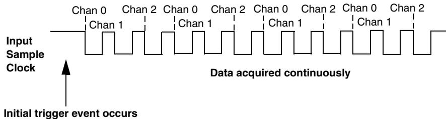
**Figure 3: Continuous Scan Mode**
