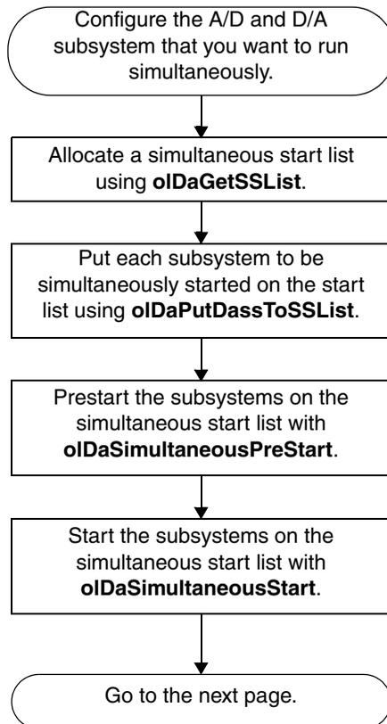
See the previous flow diagrams in this chapter; note that you cannot perform single-value operations simultaneously.
