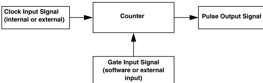
**Figure 4: Counter/Timer Channel**
