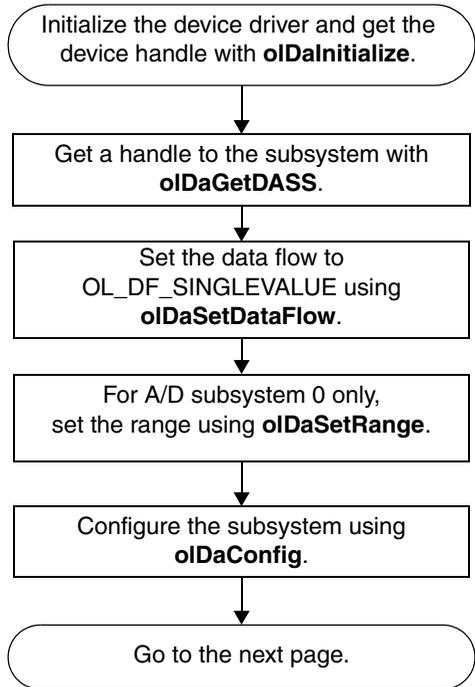
Specify A/D subsystem 0 for an analog input operation, D/A subsystem 0 for an analog output operation, DIN subsystem 0 for a digital input operation, or DOUT subsystem 0 for a digital output operation.
