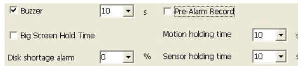
Fig 4.10 Local alarm triggering configuration
