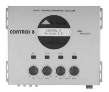
*Input Gain Controls:* Use these controls to match the pre-amp output level from your car audio source unit. Set the input level so that the SIGNAL LED (next to the input sockets) lights occasionally on musical peaks. Control8 MAX Input level: 15 V.
