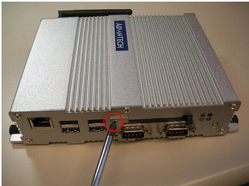
4. Unscrew the 4 hex-bolts on the front panel.
