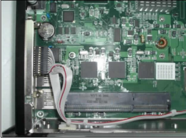
**Fig. 2-23** PCI-X slot on the back of PPAP-3720
