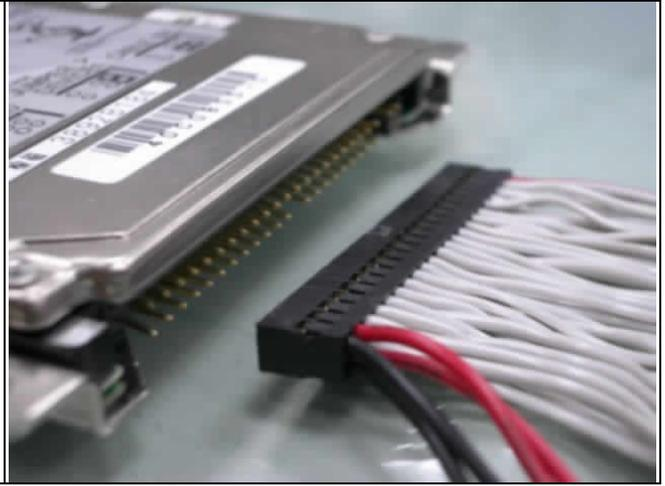
**Fig. 2-21** Connect power and IDE cable to HDD
