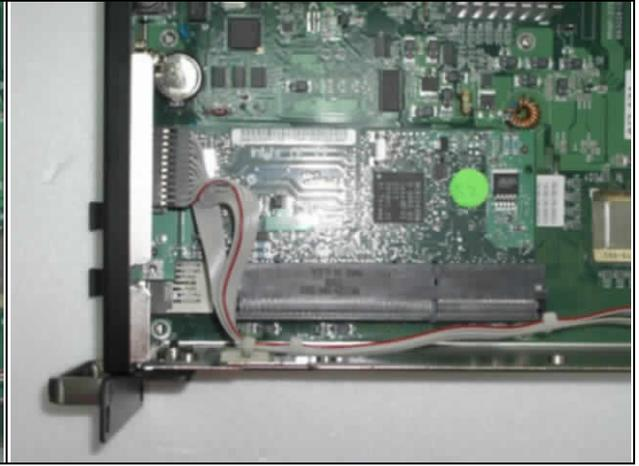
**Fig. 2-24** Push the PCI-X add-on card into the slot
