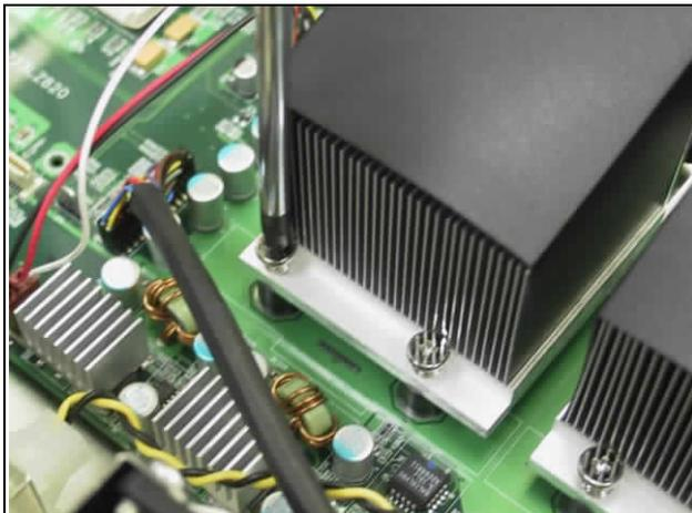
**Fig. 2-10** Loosen the screw and cpu space
