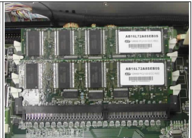
**Fig. 2-8** Install DIMM
