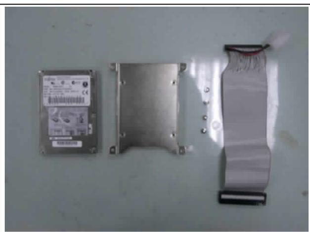
**Fig. 2-19** A 2.5" HDD and the HDD bracket
