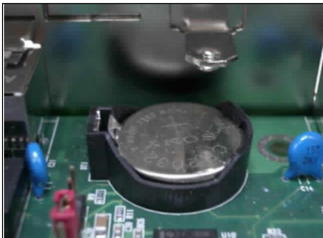
**Fig. 2-16** Eject the battery
