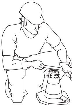
Figure 34-D. Slump Test (Removing Excess Concrete)
