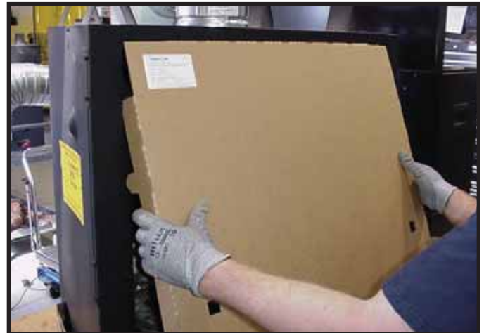
Figure 13.8 Installation of Splatter Guard
