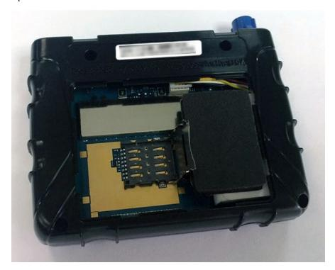
3. Insert the SIM card into the SIM holder.
