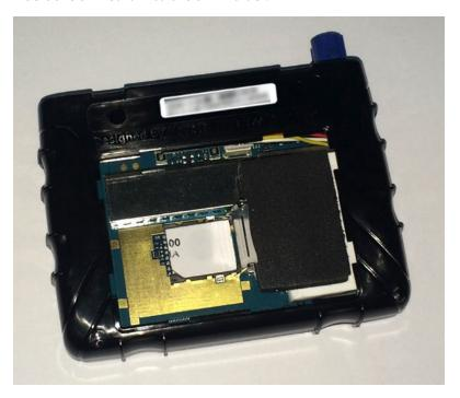
4. Close the SIM slide, the push the slide to the left and lock it down.
