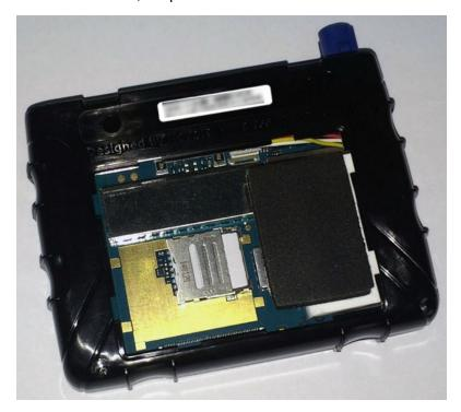
5. Insert the device "door" plate into the opening and snap into place.
