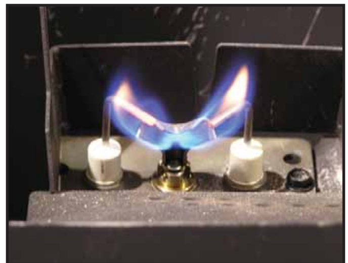
Figure 3.2 IPI Pilot Flame Patterns
