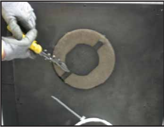
Figure 9.5 Cut the metal retaining band.
