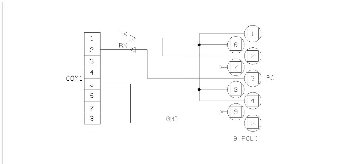
**Figure 15.1 - Connection between PC and terminal for firmware upgrade** (*citi0629.gif*)
