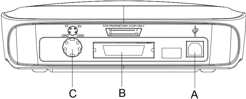
Figure: Rear view of CD-RW drive
