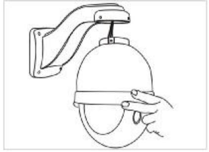
5. Make the connetion plug ,which has been connected plug into the relevant place, and then connect the flange with dome connector to make the dome being installed.
