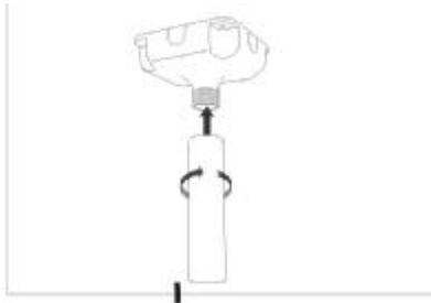
3Make the cable connection drill through the joint pole in the center of the mount,and then circumvolve the joint pole and mount place together.
