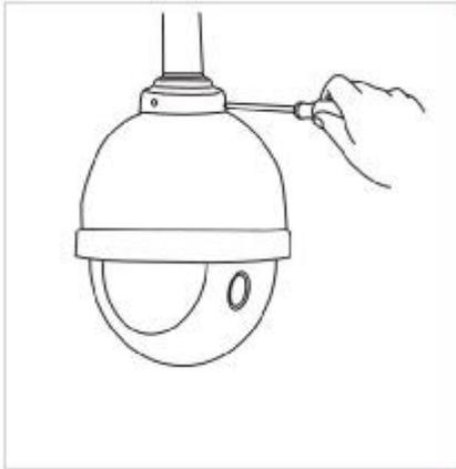
6. Take the screw out from accessory ,which used to fix the dome and the mount ,fix it with Alley Key, and then take the protection sponge and lens cap from inside dome ,setup the protocol and code in light of instruction.
