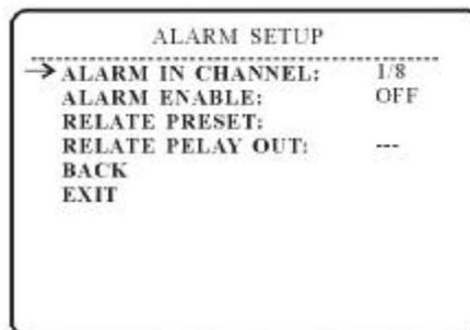
Match the Alarm sensor input to one of Preset positions.If an external sensor is activated, camera will move to corresponding preset position when this item is predefined.
