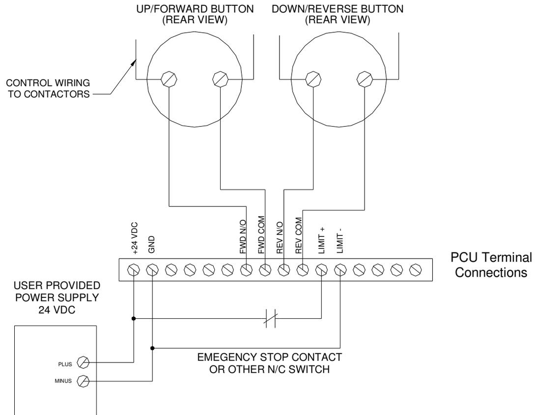
The PCU requires a user provided 24 VDC power supply to operate. In some cases, this can be derived from existing machine power, if available. If no 24 VDC power is supplied within the machine, an additional power supply will be needed. This can be either an open frame industrial power supply available from many electrical supply distributors or an optional plug-in power supply available from Accurate Technology, Inc.
