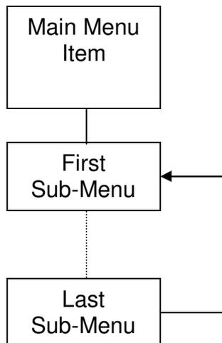
To exit from the sub-menu system, **press AND hold** the [F] key for approximately 1.5 seconds. The system will return to the top-level menu listing showing the **next** available top-level menu.
