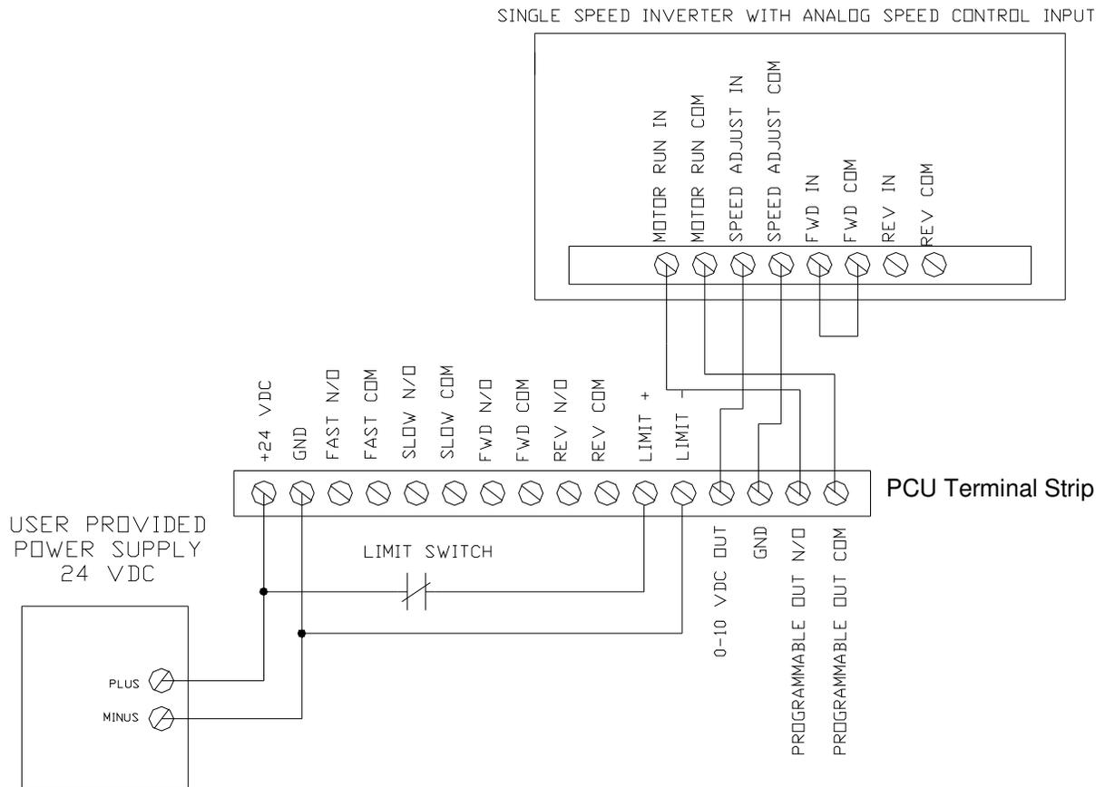
In this application, the PCU energizes a normally open relay whenever the conveyor output is to become active. An analog output voltage from 0 to 10 V DC is used to control the desired speed of the inverter.
