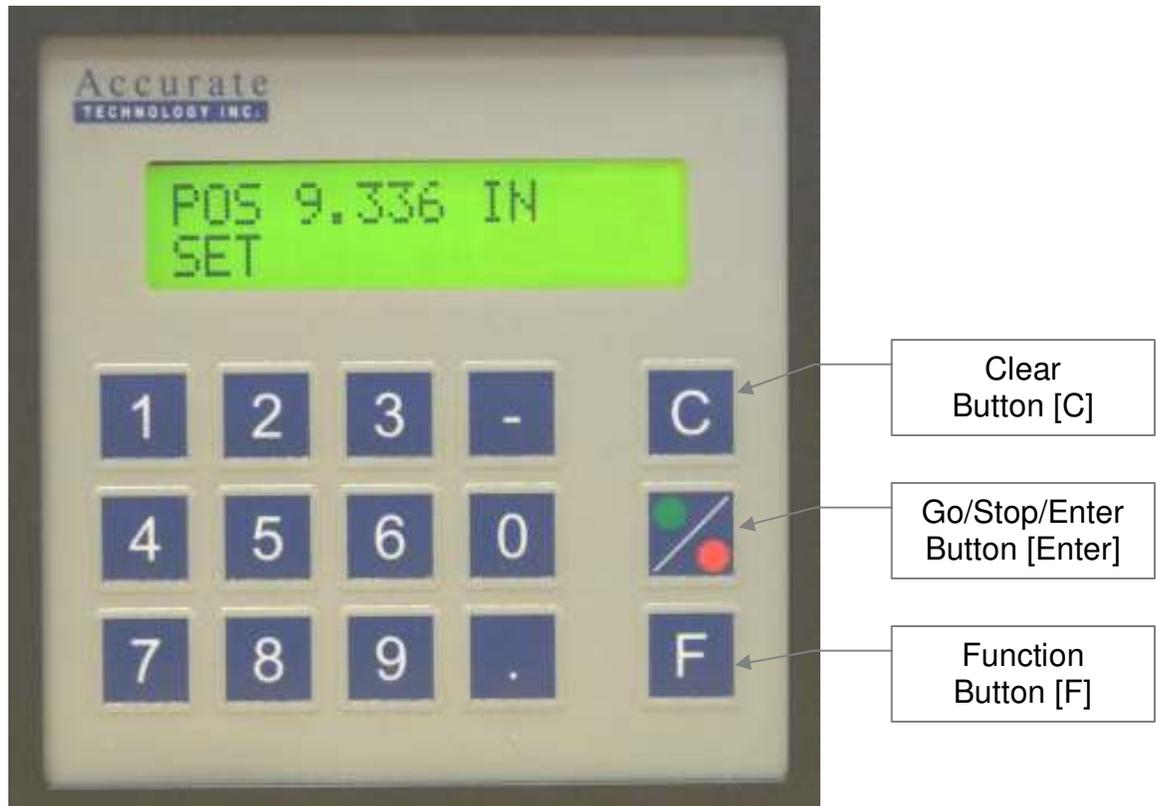
The keypad consists of a total of 15 keys, 10 numeric, minus, decimal point, Clear [C], Go/Stop/Enter [Enter] and Function [F].
