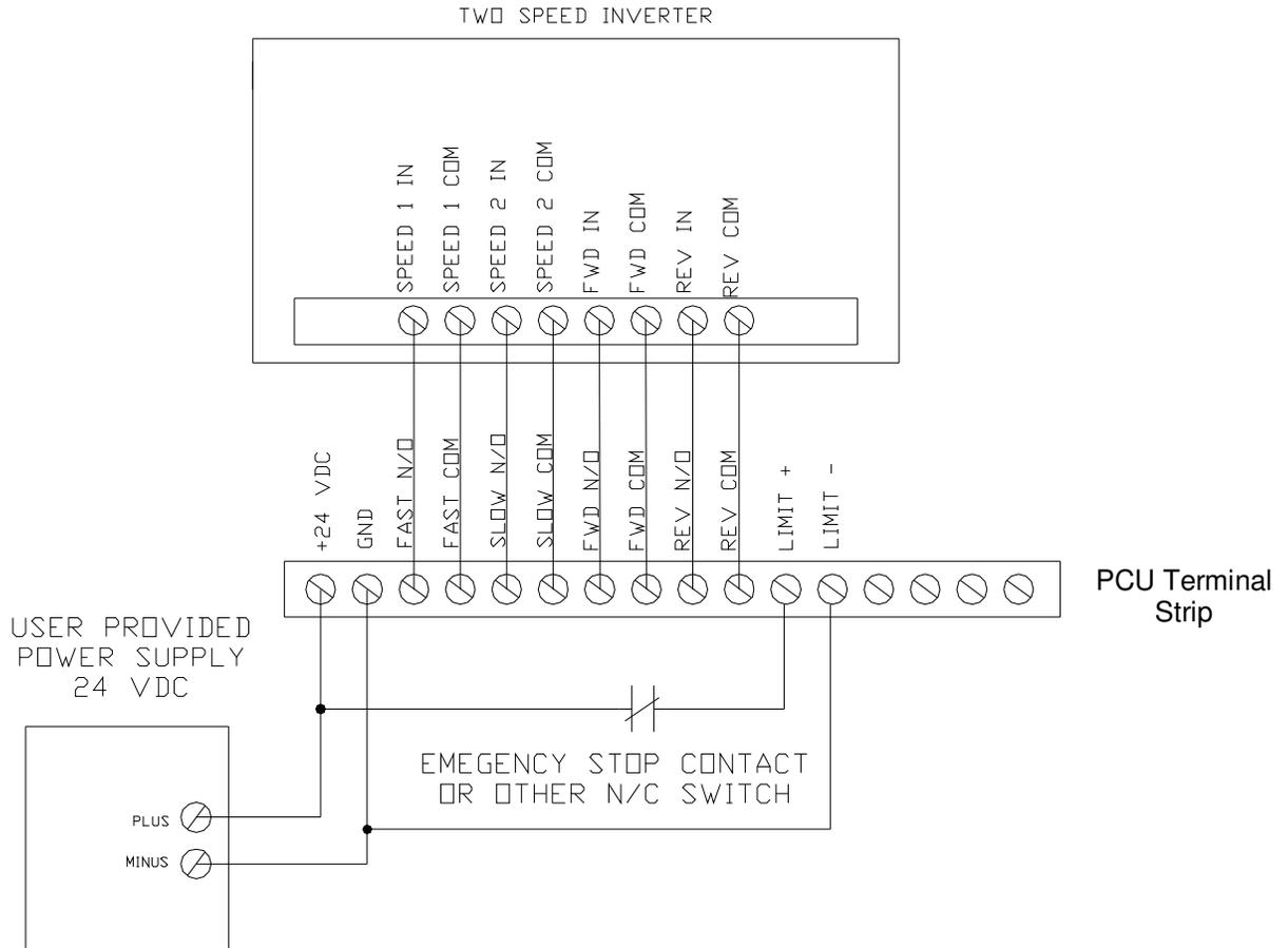
In this example, the fast and slow outputs of the PCU respectively are connected to the speed 1 and speed 2 inputs on the variable frequency inverter. The forward and reverse outputs of PCU connect directly to the forward and reverse inputs of the inverter.
