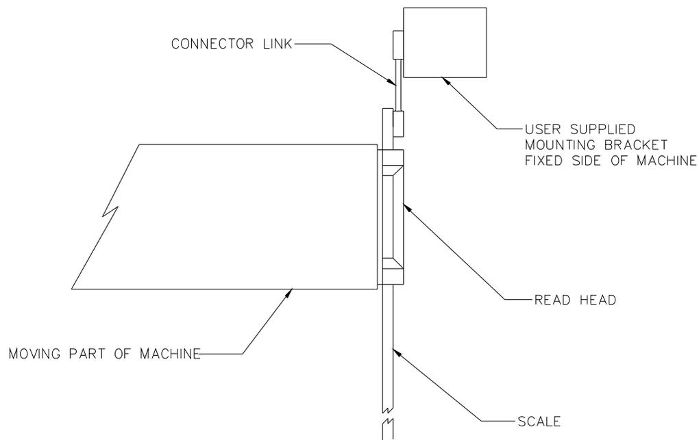
Care should be taken when installing the encoder scale and read head. To reduce excessive wear and assure accurate measurement, the encoder scale should be mounted as parallel as possible to the direction of travel.
