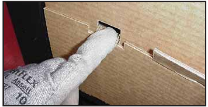
Figure 13.9 Securing Tabs Inside Front of Splatter Guard
