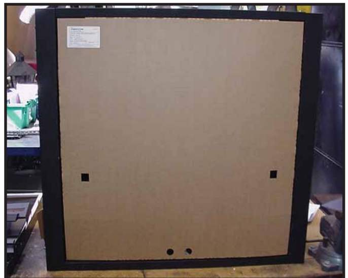
Figure 13.11 Splatter Guard with Lower Access Panel Closed
