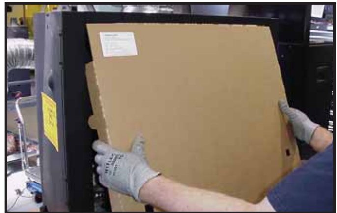
Figure 13.4 Installation of Splatter Guard
