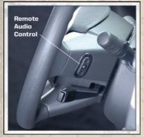
The switches are located on the rear surface of the steering wheel.
