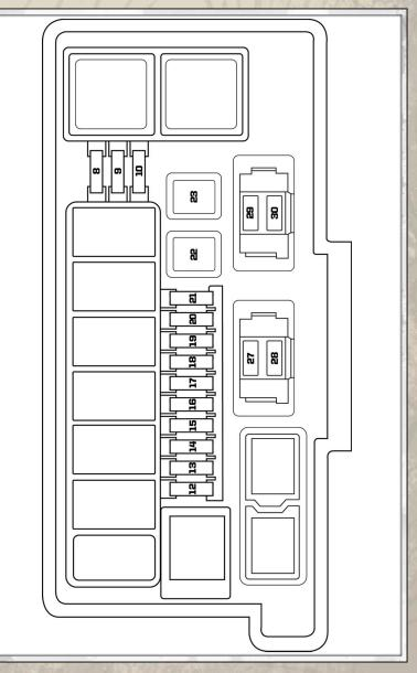
• The Integrated Power Module (IPM) is located in the engine compartment near the battery. This center contains cartridge fuses, mini-fuses and relays.
