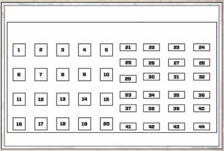
The Power Distribution Center (PDC) is located in the left side of the engine compartment near the Brake Fluid Reservoir. This center contains cartridge fuses, mini-fuses and relays.
