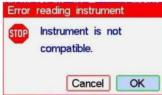
If the DL can't read the connected digital probe will be shown a dialog box:
