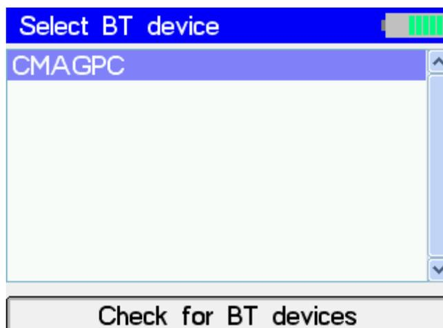
To send data to a remote BlueTooth™ device, select it in the list and press the **ENTER** key.
