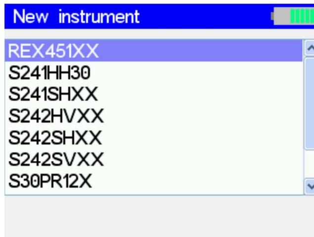
Select the probe type in the list according to your probe (probes type are listed in **Appendix A**) and press **ENTER**.
