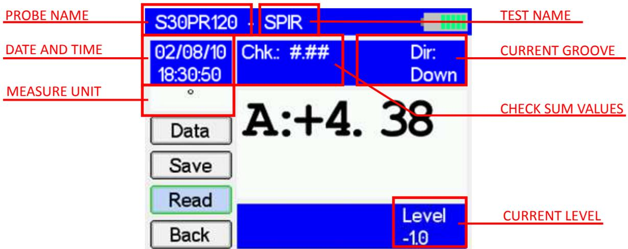
The top blue box displays the **Check sum value**; it is the halved sum of the current run and the matching run (up for down and down for up) at the current level; the readings in the matching runs should be exactly opposite, so that the check value should be close to zero; this value is only available when the matching run has already been performed.
