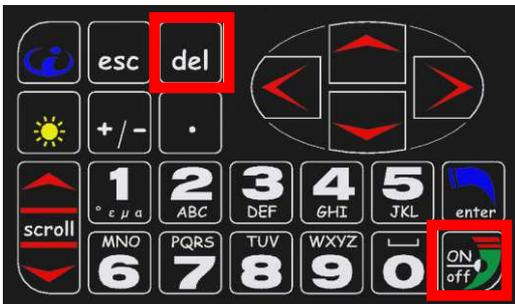
Should the DL become unresponsive, press the keys **OFF** and **DEL** keys at the same time: the DL should reset immediately.
