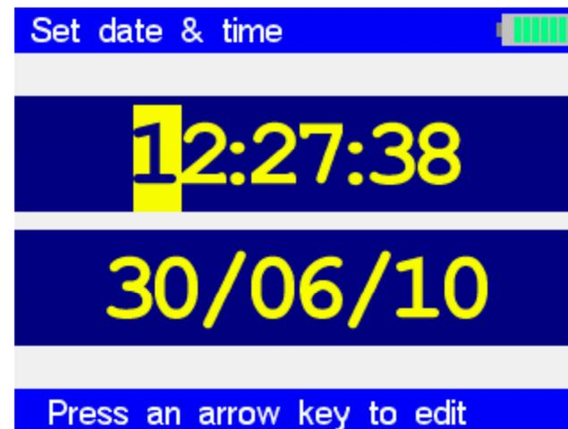
You may move the cursor using the arrow keys or change the current value by typing the new value with the numeric keys.
