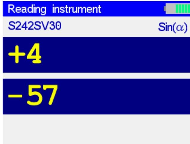
During the reading of a digital probe, pressing the RIGHT key, it is possible to display the temperature read from the probe.
