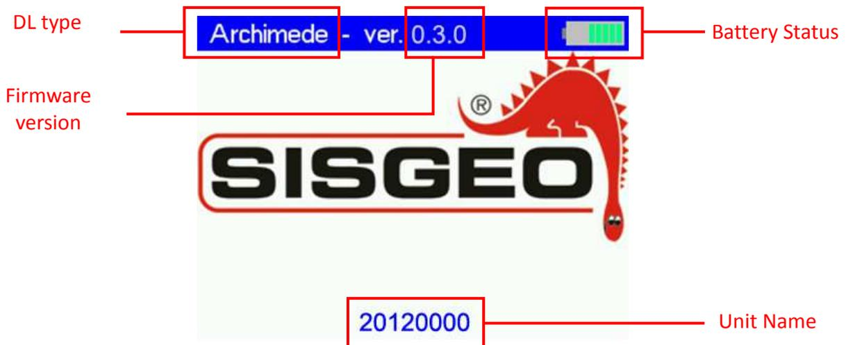
At the upper right corner the display shows the current status of the battery: the remaining charge is shown by the number of bars.
