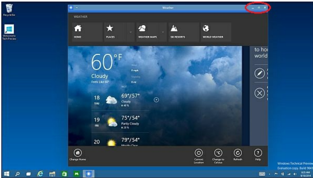
Figure 2. Modern UI apps will run on the Desktop in a window with minimize, maximize, and close boxes.
