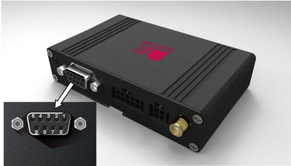
Figure 10: Pin assignment RS-232 (D-Sub 9-pole female)
