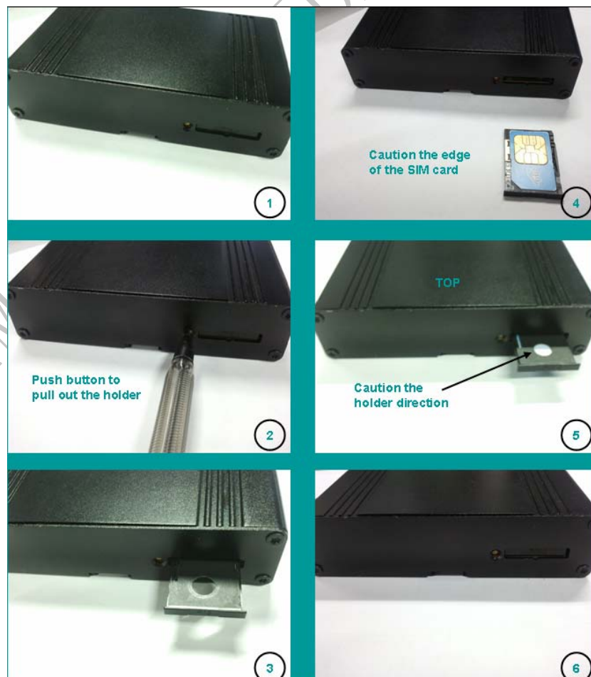
Figure 17: Installation of SIM Card
