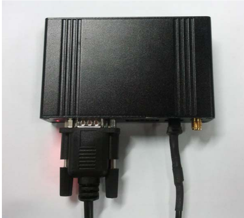
Figure 23: power up the terminal
