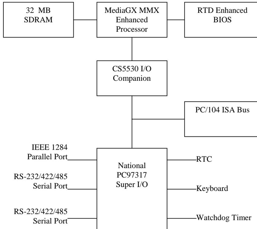
You can easily customize the cpuModule by stacking PC/104 modules such as modems, LAN controllers, or analog and digital data acquisition modules. Stacking PC/104 modules on the cpuModule avoids expensive installations of backplanes and card cages and preserves the module's compactness.
