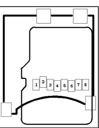
Notice that the pad numeration is written at the bottom of OLinuXino-MINI under the microSD card connector.
