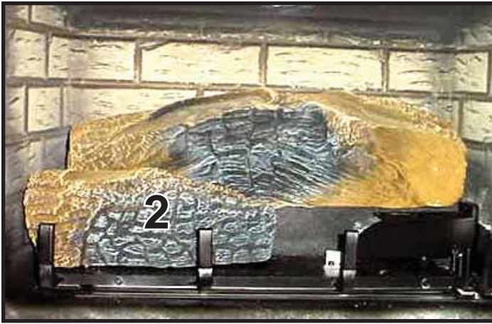
LOG #2 (SRV2019-702): Position log #2 by locating its slot over the tabs on left front of the burner.
