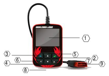
1. LCD DISPLAY -- Indicates test results.
