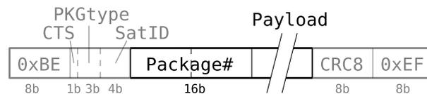
Figure B.2: Layout of a type 0 package.
