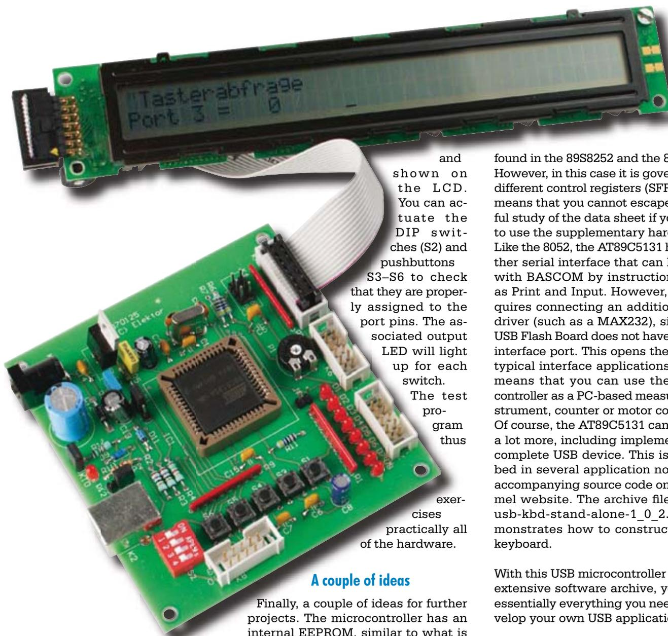
and shown on the LCD. You can actuate the DIP switches (S2) and pushbuttons S3-S6 to check that they are properly assigned to the port pins. The associated output LED will light up for each switch. The test program thus exercises practically all of the hardware.
