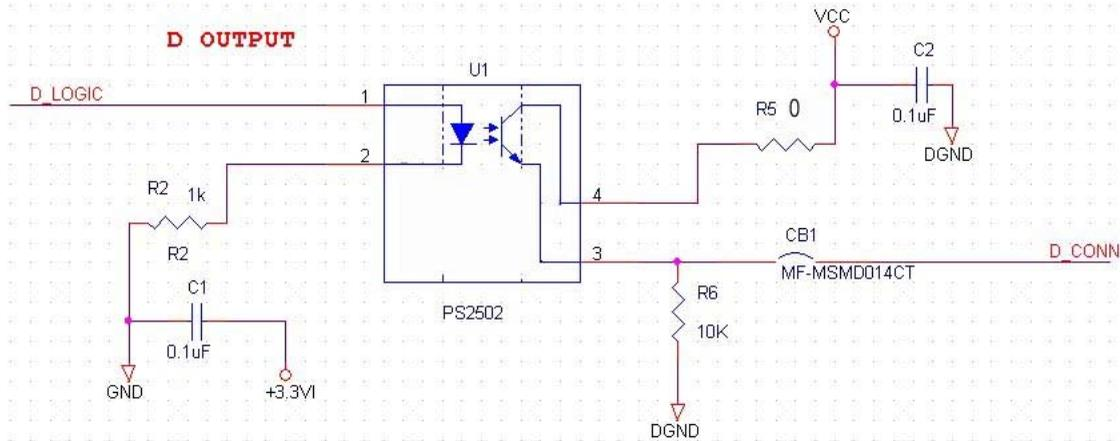
The maximum current thru the transistor should be limited to 100mA by the *CB1* fuse. User should supply *VCC* to collector of the transistor.
