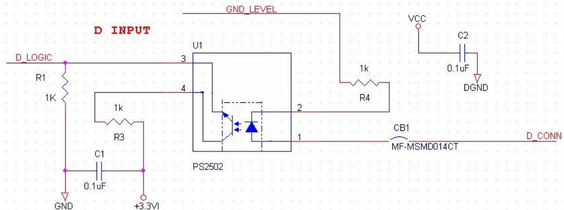
To switch input to a logical one, the user should provide current flowing through the LED in the optical isolator. The minimum current requirement is 2.4mA. The current is limited by resistor R4 and can be as high as 36mA at the maximum input voltage.
