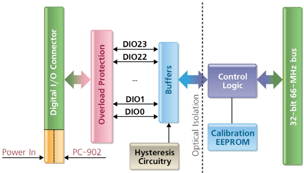
The DIO-40x layers have similar architecture. The I/O part of the layer is isolated from the logic interface via optocouplers.
