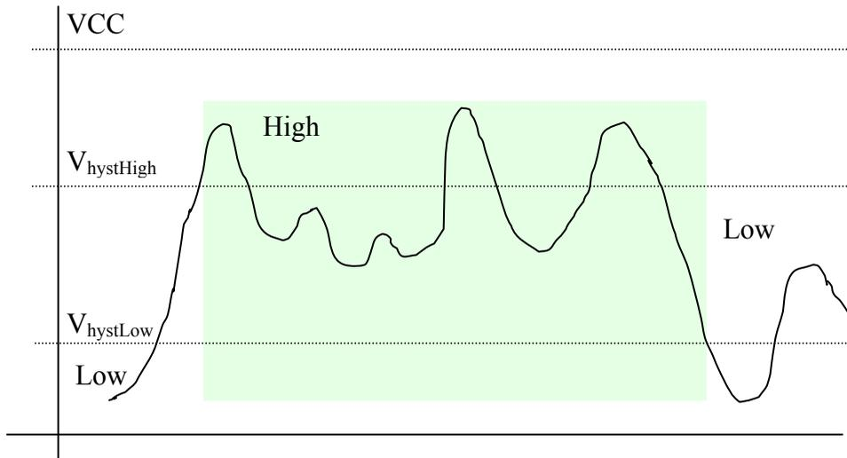
Hysteresis is a specific feature of DIO-40x layers. To access this feature, you should enable it in the configuration word:
