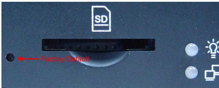
3. Power on the camera. Don't release the button during the system booting.
