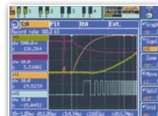
Rotary encoder output via adapter L50-Z18 connected to a measurement channel to record a fast motor start with high resolution
