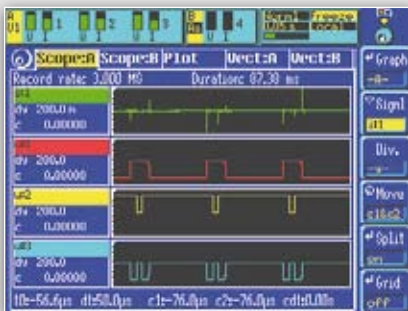
Extra-high current peaks at simultaneous switching edges
