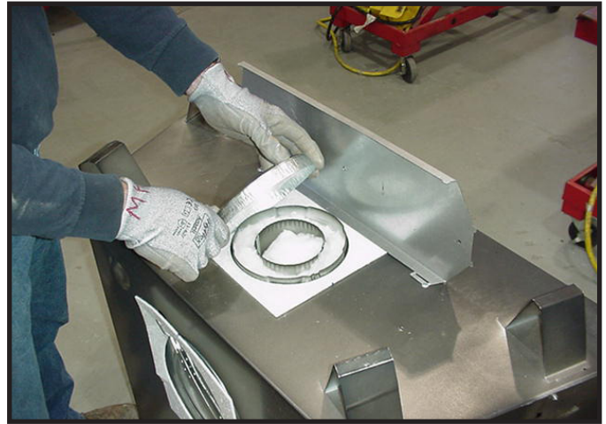
Figure 9.4 Remove the seal cap.
