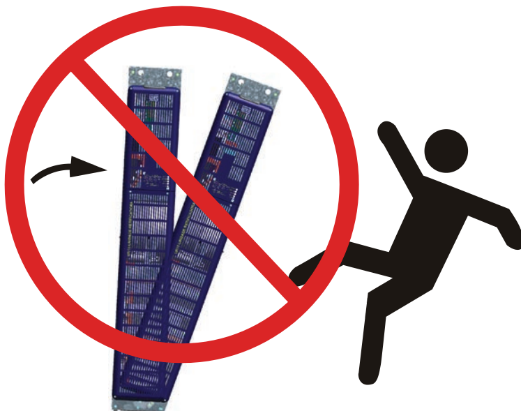
Figure 2.10 - Do not tilt the rectifier units
