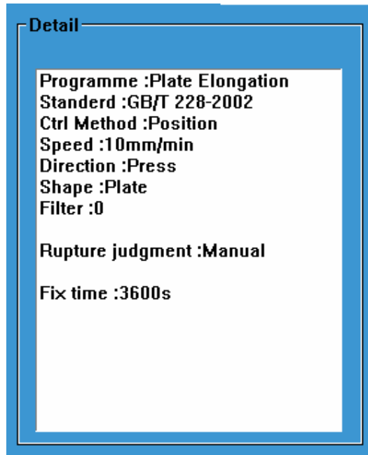
Picture (16) Details of testing scheme
