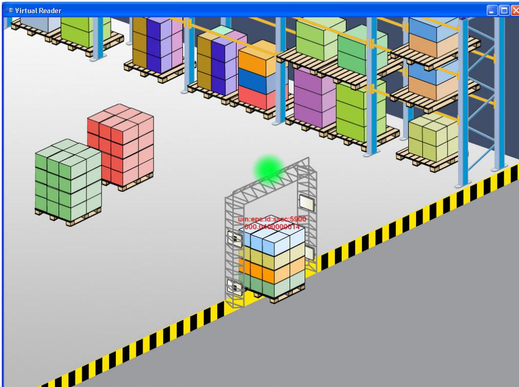
We thus see, in the warehouse, three pallets prepared for shipment: two homogeneous pallets and one mixed pallet. The readout takes place by physically moving pallets through the RFID gate using the mouse. At the same time, a small semi-transparent window shows the numbers SSCC and SGTIN of the goods read.
