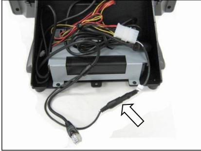
5. Tilt the unit and remove the I/O Panel cover (see arrow).
