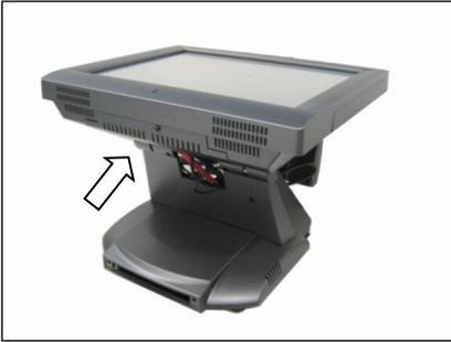
9. Cut the cable slot on back cover (see arrow).
