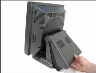
2. Install the rear display to the unit, secure it with five *Phillips M4 x 8 Big-Cap Black* (P/N: 10-S4008BB) screws.
