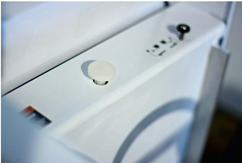
Raise the build platform several inches by turning the white knob, located in the top-middle of the build area, then remove the accessories box held underneath.
