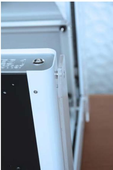
Gently lay the printer on its back to attach the acrylic side panels using the large bolts and spacers, which are placed between the side panel and printer. The panels engraved "Type A Machines" go on the top. The panels engraved "Series 1" go on the bottom.
