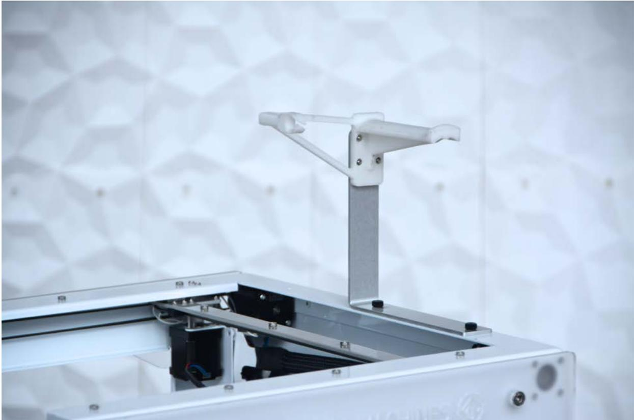
Attach the spool holder to the L-bracket with the 4 small bolts. Do not over tighten. Attach the assembly to the top of the printer using the black topped thumb screws. The spool holder should be attached so that the filament feeds forward.
