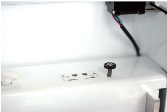
The 2014 Series 1 3D printer features a black Z height adjustment knob, shown left, at the top right of the build area. That knob is used to increase or decrease the distance between the print head nozzle and the build surface for the first layer of a print.
