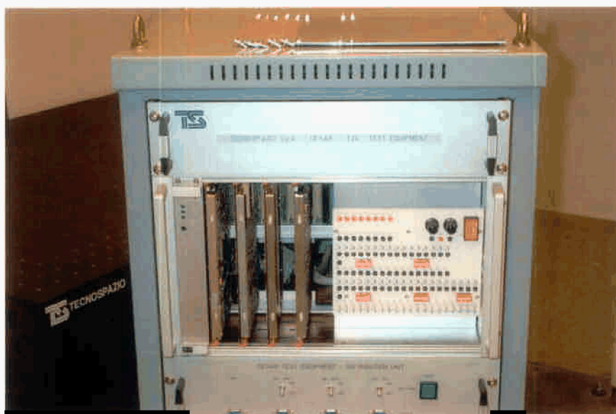
Fig. 4.1.1-1 Front view of opened VME crate
