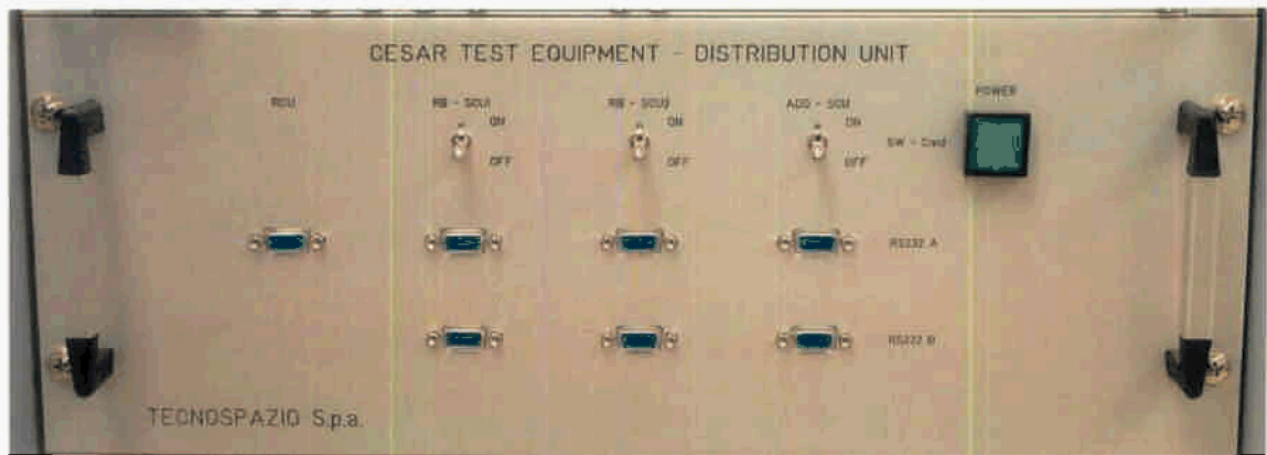
Fig. 4.1.3-1 Front view of Distribution Unit
