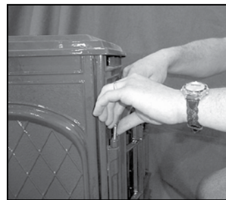
Figure 8.15 Place a washer on the top of the door hinge. Line up the hole in the door hinge and the washer with the hole in the hinge box of the face. Place a gold-plated hinge pin in the hole to secure.
