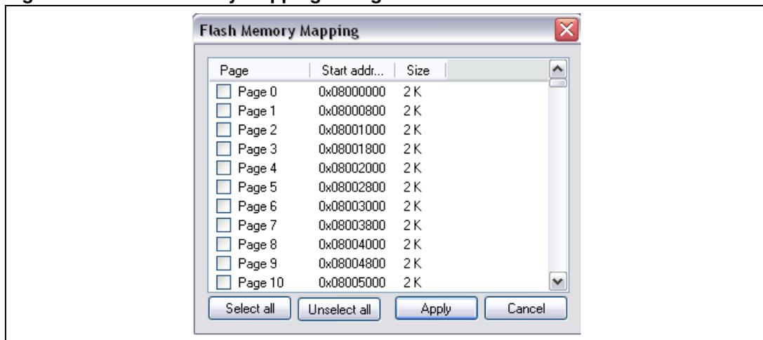
*Note:* To erase the Flash data memory sector of the ultralow power STM32 L1 devices, select the data memory box at the end of the list and click **Apply**.
