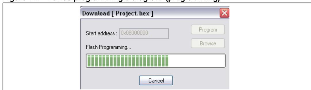
4. Finally, click on the **Program** button to start programming. If you selected **Target | Program & Verify...** in the first step, a check is done at the end of the programming operation (see [Figure 12](#)).
