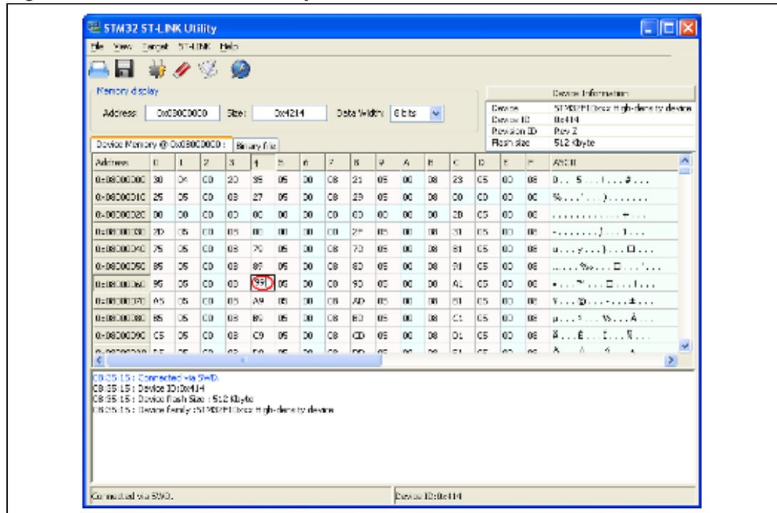
**Note:** When the Memory data zone displays device memory contents, any modification is automatically applied to the chip. You can modify user Flash memory, RAM memory and peripherals registers.
