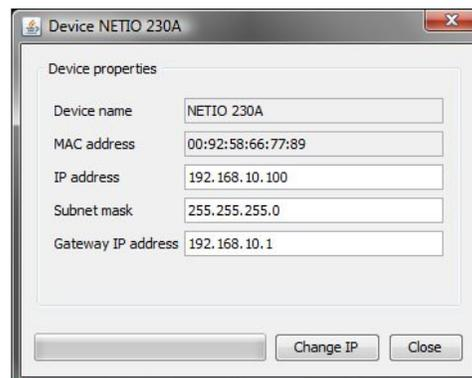
After you make requested changes based your network environment click *Change IP*. Utility will update settings of your NETIO and show device list with changed parameters. **If there is DHCP server in your network and you are not willing to setup network parameters manually, just skip to the next step.**
