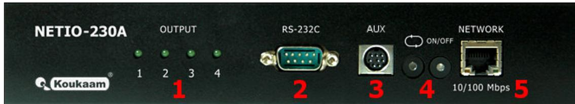
1. Four LED indicators for actual status of each outlet. If the output is ON the LED indicator shines.
