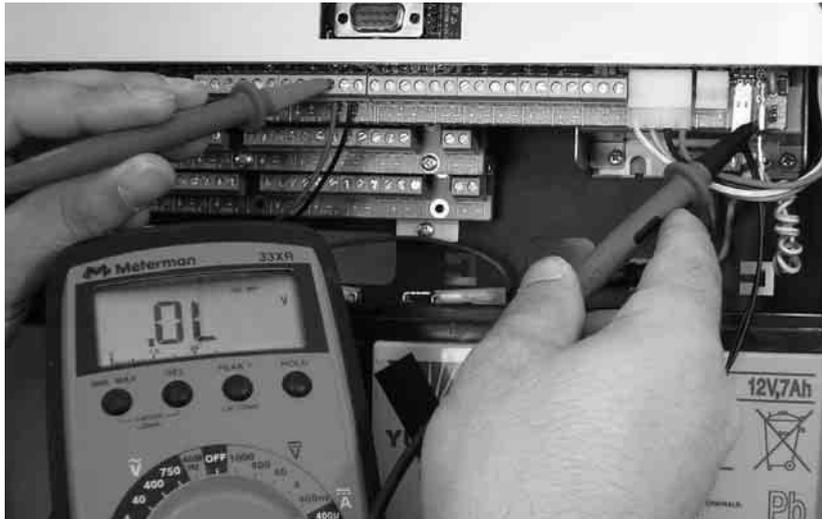
**Figure 35 - Isolation between cable shields and earthing system**
