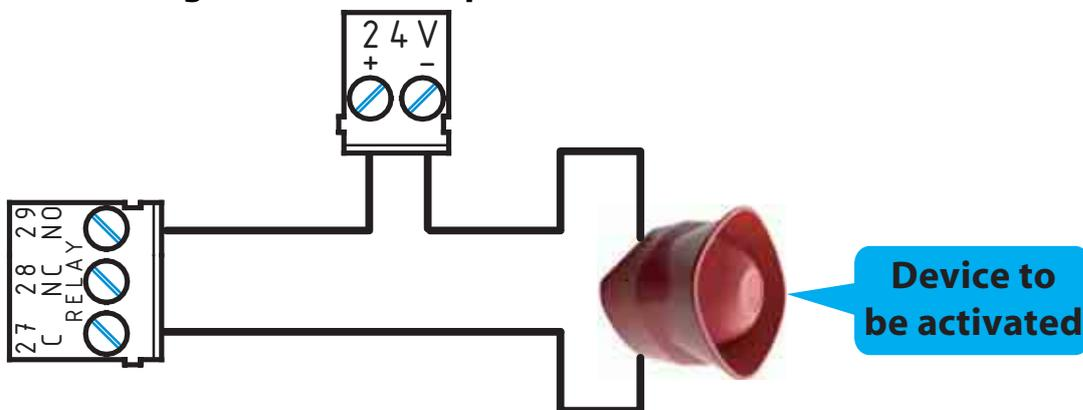
**Figure 29 - Connecting the RELAY output**
