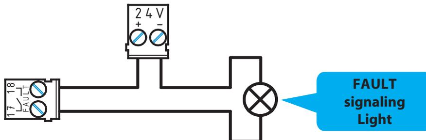
**Figure 26 - Connecting the Fault signal output**
