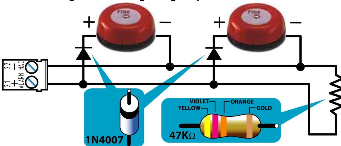
**Figure 27 - Connecting the Alarm output**
