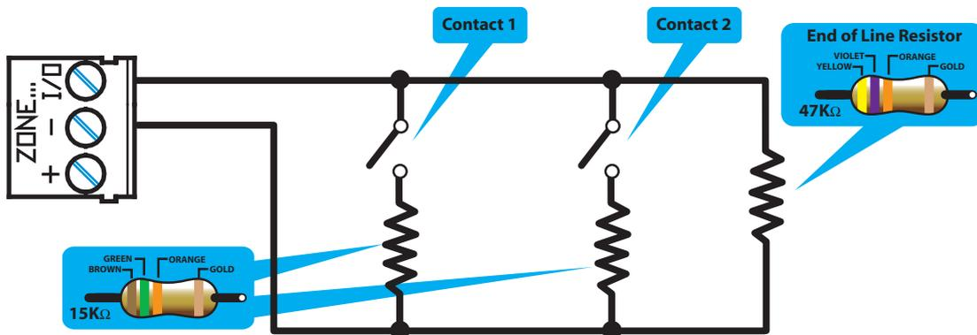
**Figure 19 - Wiring the I/O Line as an Input**
