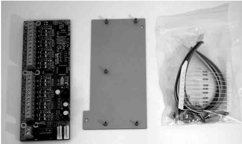
**Figure 8 - Zone expansion board - in box components**
