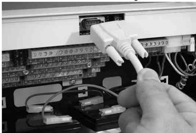
**Figure 38 - RS232 serial port connection**
