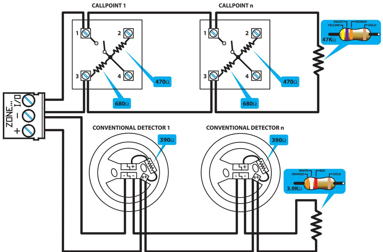
**Figure 21 - Setting up two separate lines for each zone (detectors and callpoints)**
