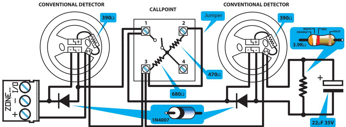
**Figure 15 - Connecting detectors using bases with diodes**
