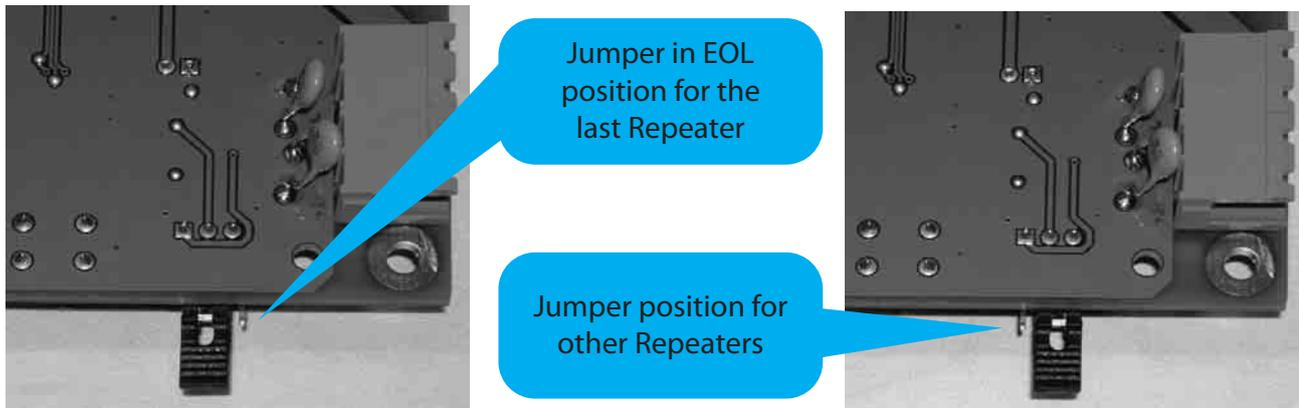
**Figure 25 - Jumper position**
