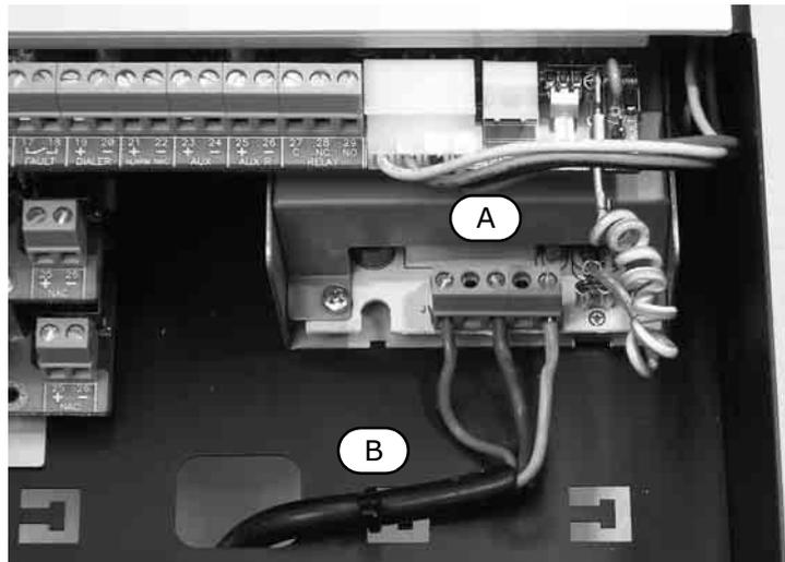
**Figure 31 - Connecting the Mains**
