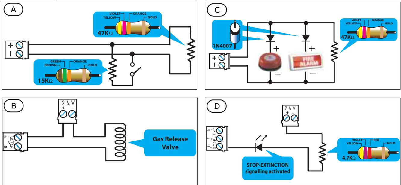
Figure 30 - Extinguishant module
