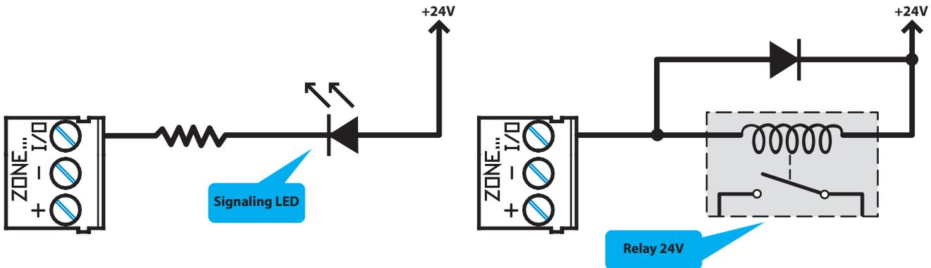
**Figure 18 - Wiring the I/O Line as an Output**
