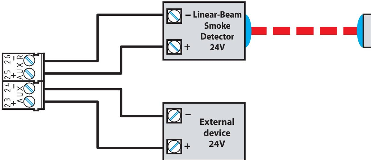
**Figure 28 - Connecting AUX and AUX-R outputs**
