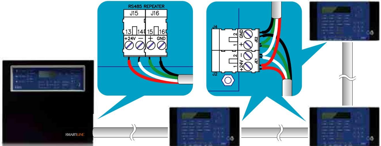
**Figure 23 - Connecting the RS485 BUS**
