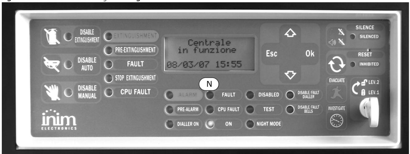
**Figure 40 - Reset signaling**
