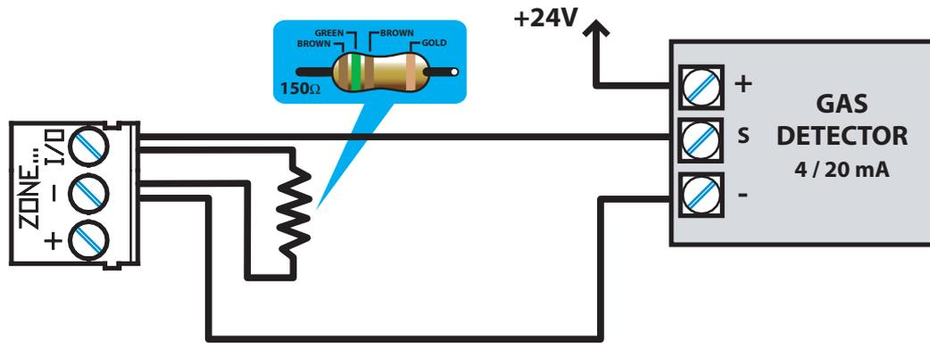
**Figure 20 - Connecting 4-20mA GAS detectors**
