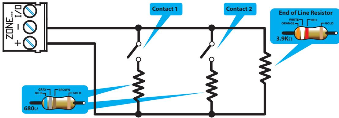
**Figure 17 - Connecting generic contacts to the detection line**
