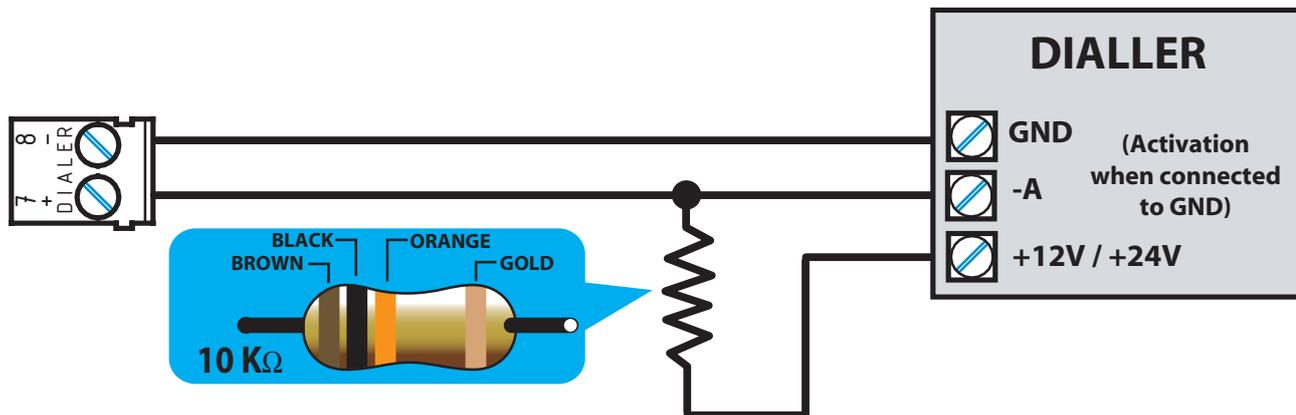
**Figure 22 - Connecting the Dialler**
