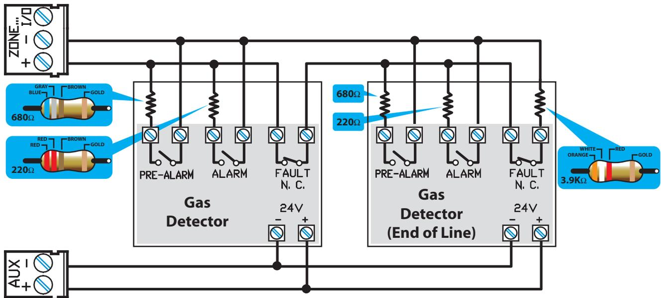
**Figure 16 - Connecting GAS detectors to the detection line**
