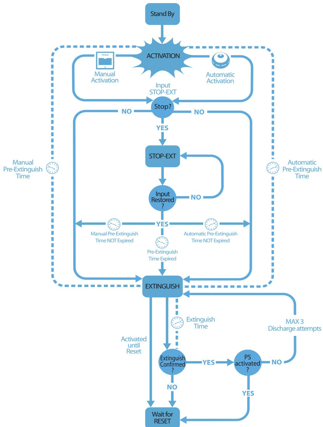
**Figure 42 - Extinguishant module: operating principles**
