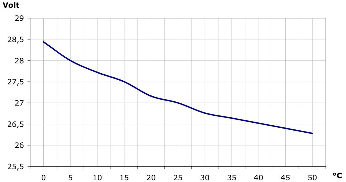
**Figure 33 - Voltage charge in relation to Battery Temperature**
