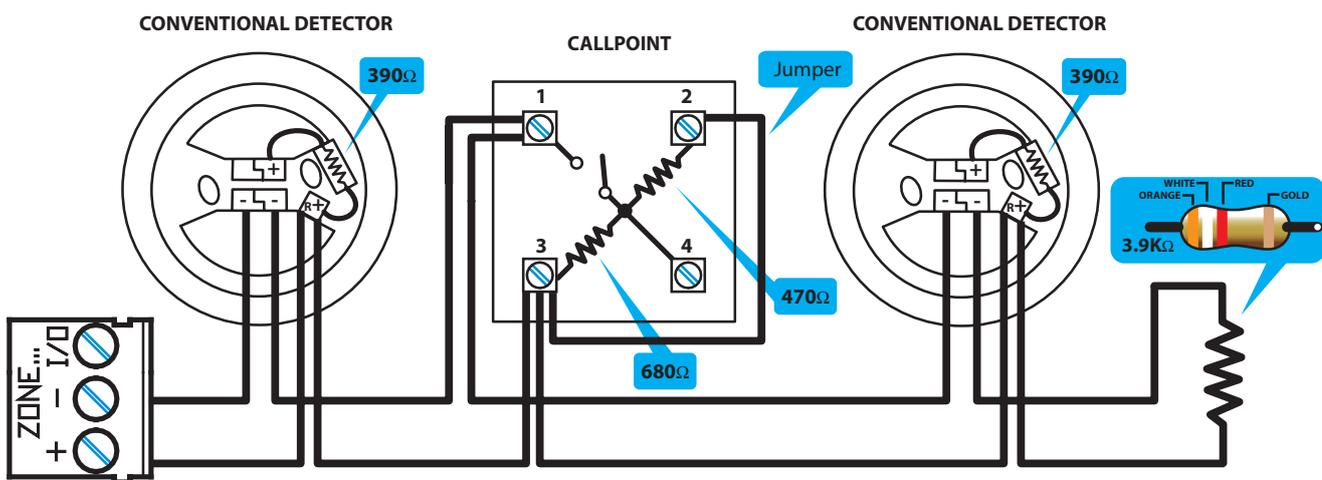
**Figure 14 - Connecting detectors and manual callpoints**
