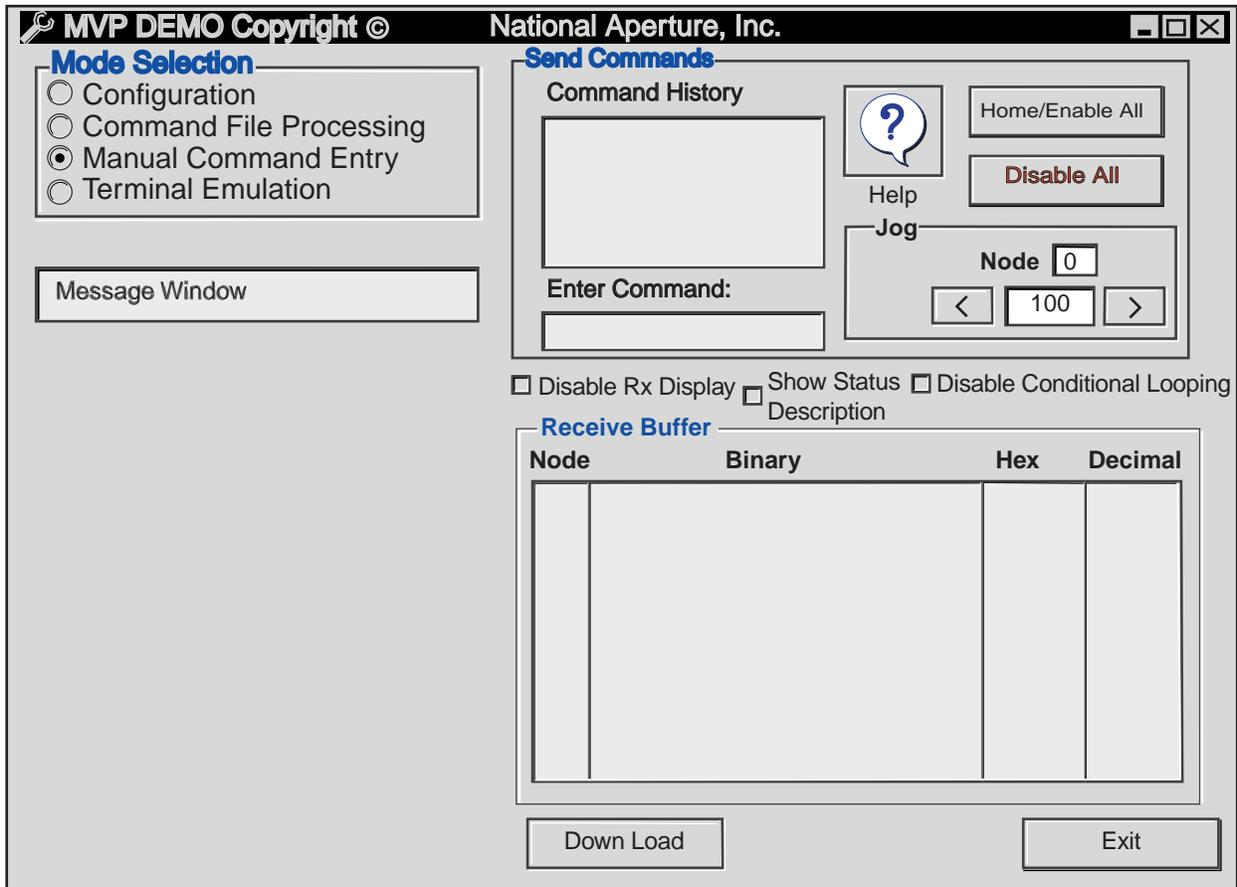
The code you will put into the “Manual Command Entry” screen will perform all functions one command at a time including any status request. It can’t be saved or edited. Each instruction is invoked only once before passing into Command History. It will, however, give you a flavor of how the command structure works and will allow you to control a servo motor. But first you will need to know a few generic motion command formalities. (See “Examples & Explanations”, next page.)
