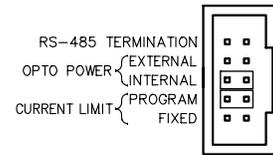
Unless you have specified otherwise, your MicroMini™ Controller unit has been shipped without a termination jumper. In the event you were to use a jumper (typically for very lengthy runs of networked modules), it is advisable to insert the jumper on the MicroMini™ Controller module furthest from the host controller. This keeps the signal levels balanced across the network. Each MicroMini™ Controller has an internal 120 Ohm termination resistor included for this purpose.
