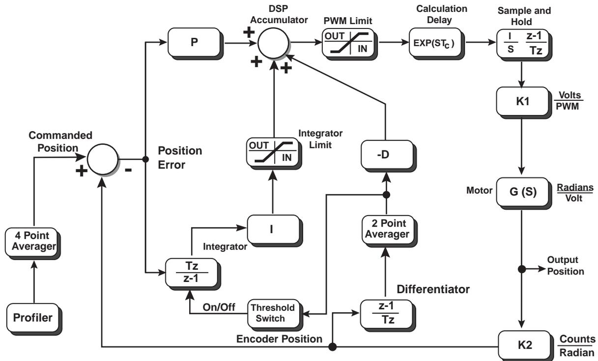
The default parameters for the digital filter have been calculated to provide stable operation in most applications. It should not be necessary to adjust the derivative term. In many cases, especially when using small, high speed motors, the proportional and integral terms are set to relatively low values and should be increased to provide the desired system response.
