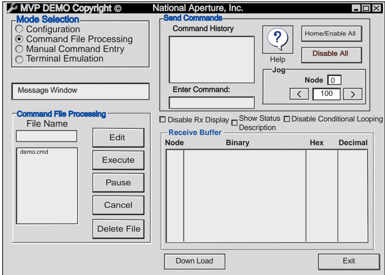
In order to construct, store, edit and execute motion routines, you must go into the programming screen by selecting the "Command File Processing" button from the Mode Selection box. Here is what it looks like.
