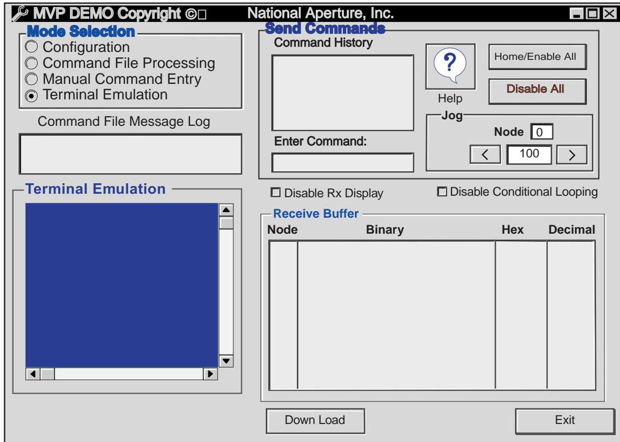
Terminal emulation mode allows direct interaction with the MicroMini™ Controller. Command strings entered in terminal mode are sent directly to the target controller and response data is displayed in the terminal window. Configuration for terminal mode is the same as for all other modes. This provides a means to troubleshoot communications difficulties without the overhead of additional software.
