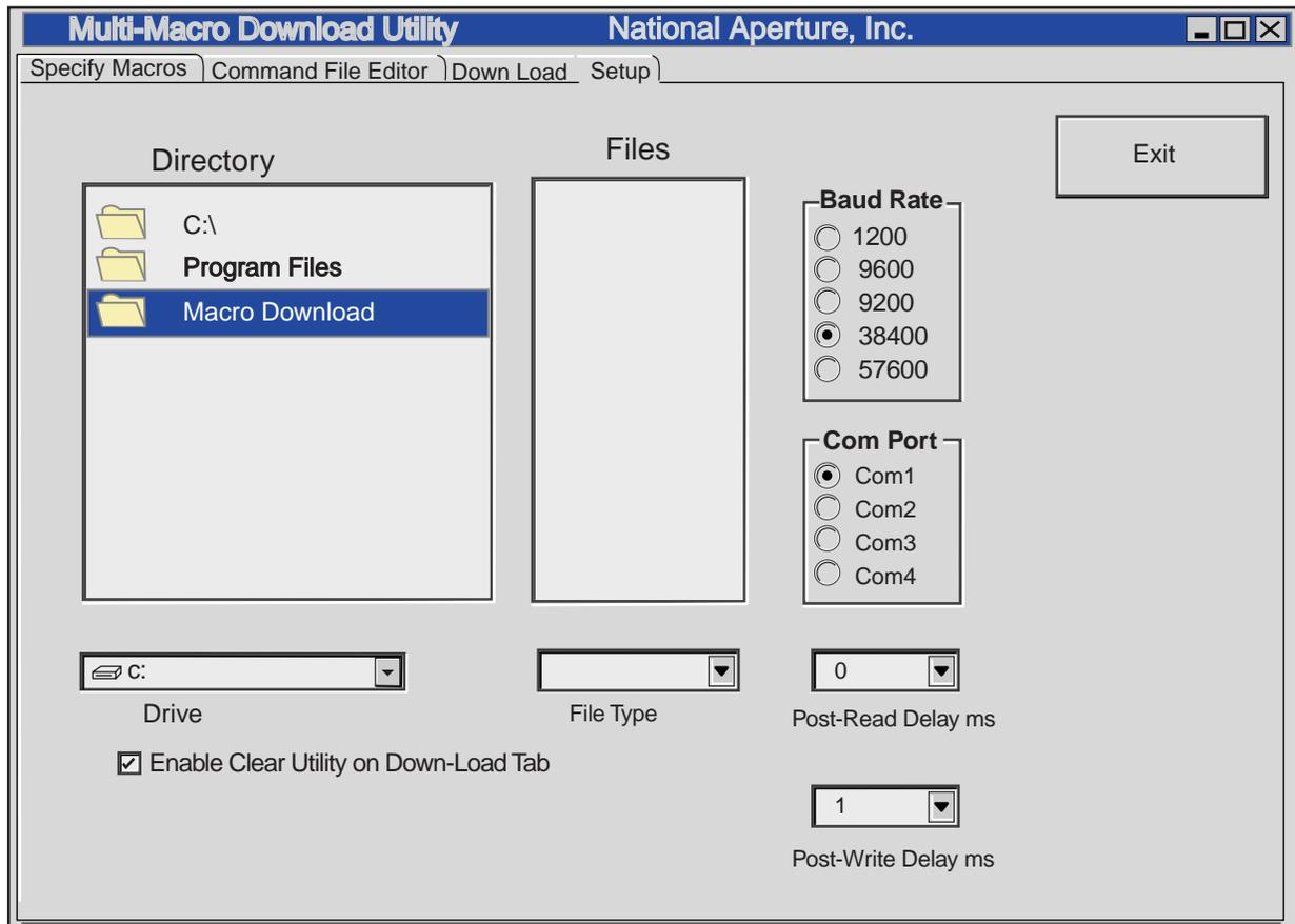
In the Setup screen, select the disk drive desired, the baud rate, and the serial com port you wish to use when downloading macros to the Macro Module. Initially set the 'Post-Read Delay' to 0 and the 'Post-Write Delay' to 1. The program will retain these settings until you change them in the future.
