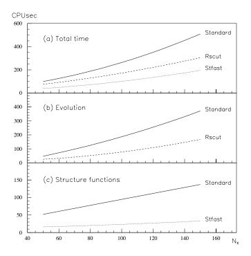
Figure 3: CPU time spent for 2500 evolutions and 250000  $F_2$  calculations as function of the number of x-grid points for a 60 point  $Q^2$ -grid. (a) Total time; (b) time spent in QCD evolutions; (c) time spent in structure function calculations. The dashed curves correspond to evolutions on part of the grid and the dotted curves to invoking fast structure function calculation in addition.
