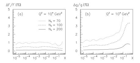
Figure 2: (a) The deviation  $\Delta F_2/F_2$  and (b)  $\Delta xg/xg$  at  $Q^2 = 10^4$  GeV<sup>2</sup> as a function of x for a 70, 100 and 200 point x grid and a 60 point  $Q^2$  grid. The deviations are taken with respect to parton distributions evolved on a  $400 \times 60 \ x-Q^2$  grid.
