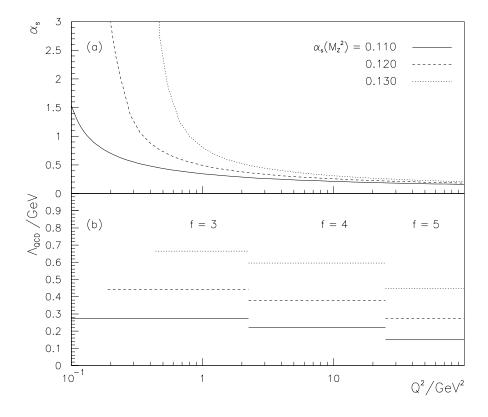
Figure 1: (a) The evolution of  $\alpha_s$  in NLO in the  $\overline{\rm MS}$  scheme starting from  $\alpha_s(M_Z^2)=(0.110,0.120,0.130)$  with the quark mass thresholds taken to be  $m_{c,b}=(1.5,5)$  GeV. (b) The corresponding values of the QCD scale parameter  $\Lambda$ .
