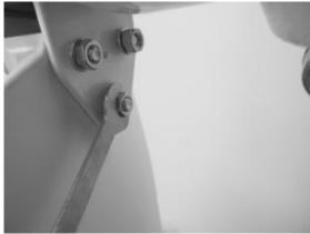
**Step 4**: Fit the nose cone onto the hub properly.
