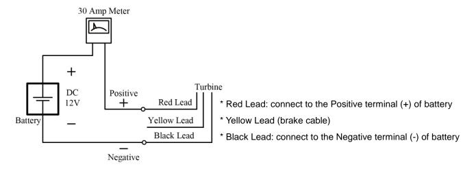
**Step 1** Disconnect the Red lead from the positive terminal of a battery.
