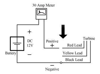
Step 2 Connect the Red lead to the Yellow lead. The turbine should be stopped immediately.
