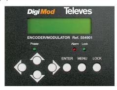
**LCD Display** – It presents the selected menu screen and the parameter settings. The backlight in the display is on when the power is applied.
