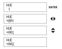
Press it to activate the hidden selections and change the setting with Up and Down (or Left and Right) buttons.
