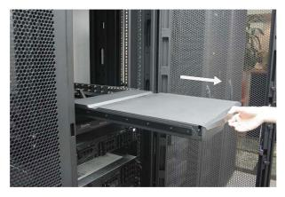
**Figure 1.** Sliding out the LCD keyboard drawer by pressing the carry
